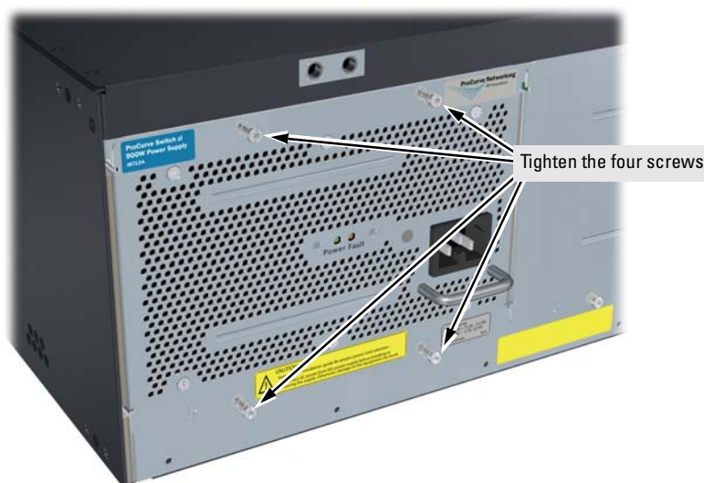
Figure 4. Fully installed power supply
